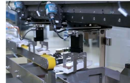
Zimmer Grippers mounted on multicarrier system movers with IO-Link Wireless Bridge
